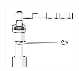
Remove the pull up rod tool (113-030-015) and install the top cap assembly. Screw the top cap onto the rod joiner and torque to 20Nm using a 12mm Socket.
