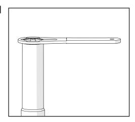
Remove the top cap from the outer tube using the top cap tool (113-010-060)
