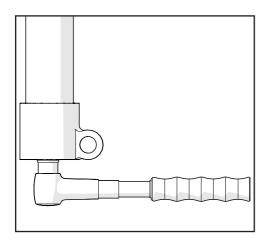
Install the base valve into the fork bottom. Torque the base valve to 40Nm using a 7mm allen key.
