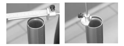
14. Refill the forks with oil and set to the recommend level using Tool No:-113-030-050 Oil Level Tool (see FF Piston Kit / FCV Application List).
