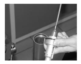
16. Before fitting the top caps screw the rebound adjustment screw fully anticlockwise and the back in four full turns. The amount of clicks per revolution may differ from fork to fork.
