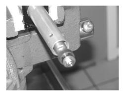
6. It is now possible to remove the piston rod out of the bottom of the cartridge tube.
