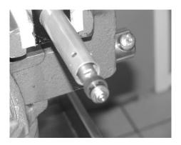
11. Refit the newly assembled piston rods back into the cartridge tube.
