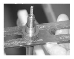
15. Before fitting springs and top caps make sure the top cap locking nut is screwed down fully onto the piston rod.
