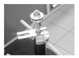
3. Remove top cap, spacer, spring using Tool No:- 113-040-010
