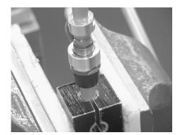
5. Remove hydraulic lock assembly on the damper rod on the cartridge that has been removed from the fork leg (screwed together type) you need to clamp the piston rod with Tool No:- **113-050-010**. Split the collar using a 19mm spanner and 17mm spanner, remove circlip from under the assembly and slide it off the piston rod.
