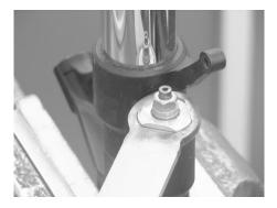
13. Remove compression adjuster assemblies and fit the new assemblies supplied with the piston kit
