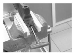
3. Clamp the cartridge tube using Tool No:- **113-070-020** and remove the base valve assembly from the bottom of the cartridge.
