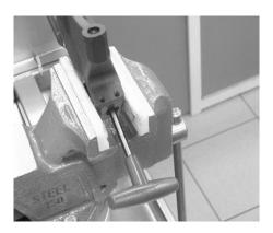
5. Refill the forks with oil and bleed any air out of the cartridge pumping the piston rod up and down. Set to the recommend oil level with tool Part No: 113-030-500. From Piston Kit Application Sheet
