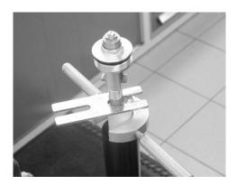
2. Remove lower bolt from axle bracket at bottom of fork and remove damping cartridge from fork and drain oil from fork.
