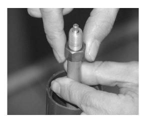
8. Screw the rebound adjustment screw on the top cap fully anticlockwise and then back clockwise four full turns. The amount of clicks may differ from fork to fork.
