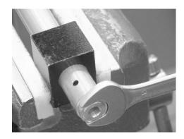
4. The cartridge is now ready to refit into the fork casing using the original bottom bolt.
