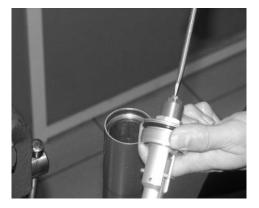
10. Refit the springs using tools Part No: 113-040-010.
