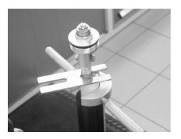
2. Remove lower bolt from axle bracket at bottom of fork and remove cartridge from fork and drain oil from fork.
