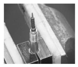
2. Fit the new rebound piston assembly to the piston rods using Loctite 243. Using the 113-050-010 piston rod clamp clamp to tighten.
