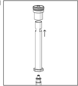
Remove the Top cap and preload spacer from the K-Tech cartridge. You are now ready to fit the K-Tech cartridge.
