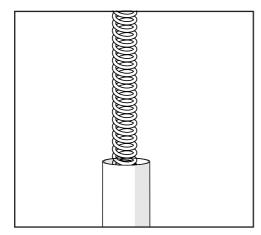
Install the chosen spring into the fork leg.
