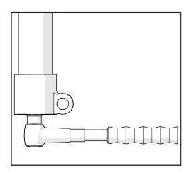
Install the base valve into the fork bottom. Torque the base valve to 35Nm using a 19mm socket.
