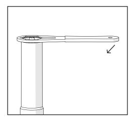
Screw the top cap back onto the outer tube but do not tighten up.
