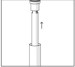
Remove the standard cartridge from the forks by pulling the top cap up and out of the forks.
