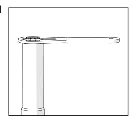
Remove the top cap from the outer tube using the top cap tool (113-010-032)
