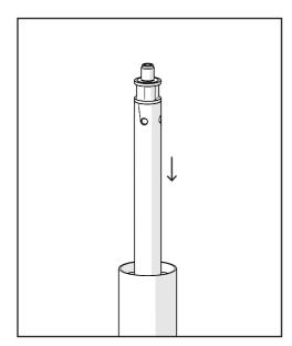
Install the K-Tech cartridge into the fork tube.
