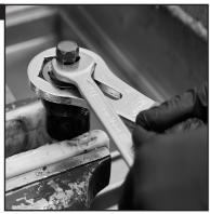
1: Remove the compression valve assembly from the cartridge assembly using cap using spanner 113-010-032 and valve assembly tool 113-010-115.
