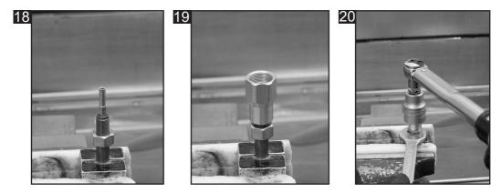
18:Hold piston rod in vice using tool 113-050-010. Install adjuster rod into piston rod.
