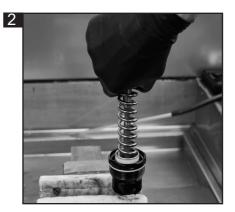
2: Remove compression valve assembly from the cartridge assembly. Hold in vice using valve assembly tool 113-010-115.
