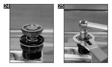
24: Screw compression valve assembly into cartridge.
