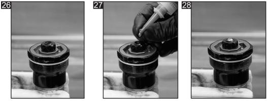
26: Install compression adjuster knob onto brass hex adjuster 27: Apply Loctite 243 to compression adjuster knob screw and install as shown.
