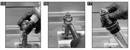
15: Apply Loctite 2701 to new rebound valve assembly thread and insert into piston rod.
