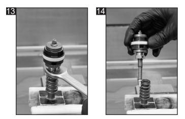
13: Hold the piston rod in a vice using tool 113-050-010.
