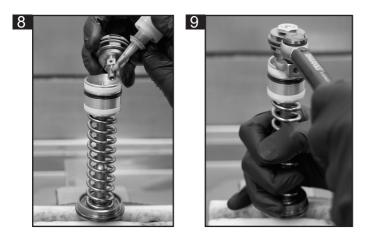
8: Apply Loctite 2701 to new compression valve assembly thread and fit into top cap rod.
