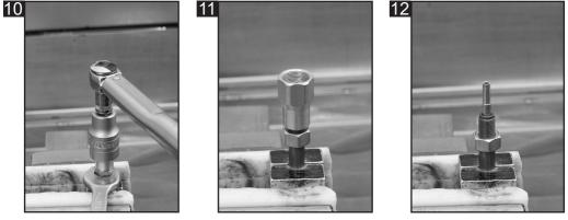
10: Remove the rebound piston rod assembly form the cartridge tube. To do this hold the piston rod using tool 113-050-010 in a vice and loosen the lock nut from the locator hex.
