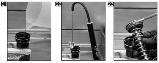
21: Fill cartridge to within 100mm of the top with 117-017-001 fork oil. Bleed the system by moving piston rod up and down around 10 times.
