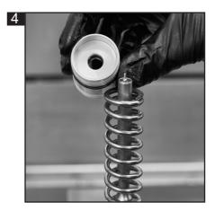
4: Remove seperation piston, pressure spring and spring seats.
