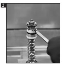
3: Remove compression valve assembly using13mm spanner.
