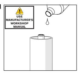
Pour in fork oil to level recommended by manufacturer. You may need to pump the fork up and down whilst doing this to allow the oil to settle.
