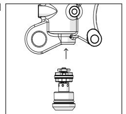
Reinstall piston rod assembly into cartridge and reinstall spring guide onto rod. Insert cartridge into fork tube ensuring it seats correctly on the fork bottom.
