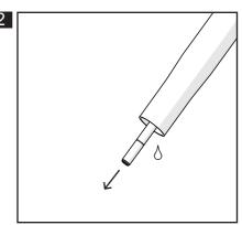
Empty the oil from the fork. Remove the base valve assembly form the fork foot using a 17mm allen key. Remove the cartridge from the fork outer.
