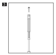
Unscrew the spring guide from the piston rod and remove the piston rod assembly from the cartridge tube
