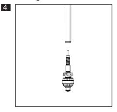
Remove the compression and rebound pistons from the piston rods. Install to both piston rods the K-tech rebound piston assemblies and needles as shown using grease on o-rings and Loctite 2701 on thread.
