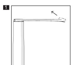
Remove the top cap from the outer tube and disassemble from piston rod.
